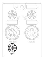
01. Connect the M12 connector to the PDCT port. See the connections below.
