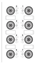
01. Connect the M12 connector to the I/O port. See the connections below.
