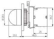
■ L2RR-L2 M (extended horn head, modular type block)
