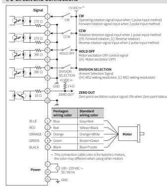
01) If the external signal input voltage is exceed the +5 VDC=, connect a resistor at outside
