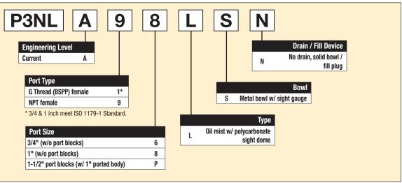
Note: All configured BSPP ported units are supplied using NPT ported bodies and BSPP port block kits.
