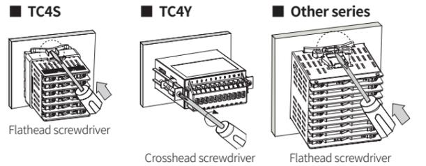
Mount the product to panel with bracket, push it to arrow direction by using screw driver.
