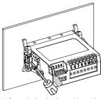
Insert the unit into a panel, fasten the bracket by pushing with tools with a flathead screwdriver.
