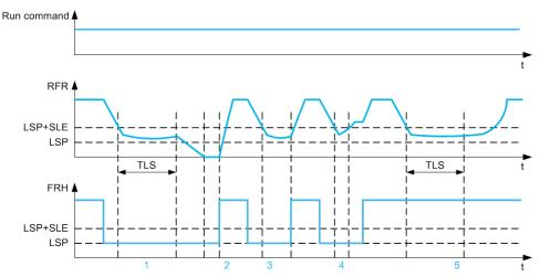
**1** Nominal **[Low Speed Timeout]** *L L* **5** function action: after **[Low Speed Timeout]** *L L* **5** time, the motor is stopped according to the current deceleration ramp
