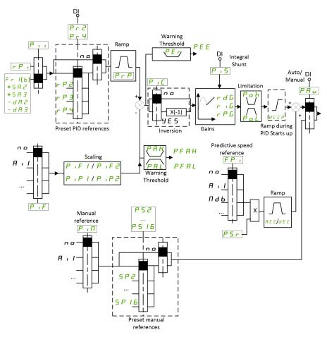
The PID feedback needs to be assigned to one of the analog inputs AI1 to AI5 or a pulse input, according to whether any I/O extension module has been inserted.
