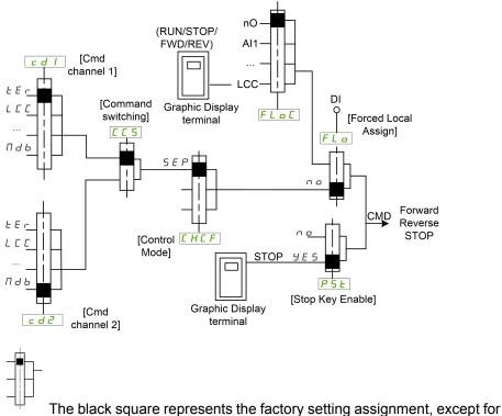
**The black square represents the factory setting assignment, except for [Control Mode]** *[ H [ F*. [Cmd channel 1] [ ] I and [Cmd channel 2] [ ] Z : Terminals, Plain Text Display Terminal, fieldbus module
