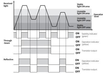
In Dark ON mode, the waveforms are reversed.
