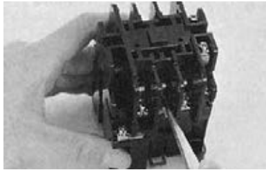
Pull out the moving contact with tweezers.
