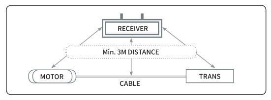
9. Install receiver top outside of electrical control box and installation in inside the control box is not a proper method.
