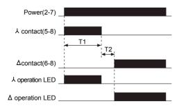
$\times$ T2:  $\lambda$  - $\Delta$  switching time ( $\lambda$  contact and  $\Delta$  contact are OFF simultaneously at power ON)
