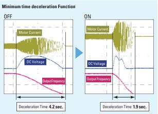
**2.3 sec. reduction of deceleration time** without a braking resistor is achieved when the function is active.
