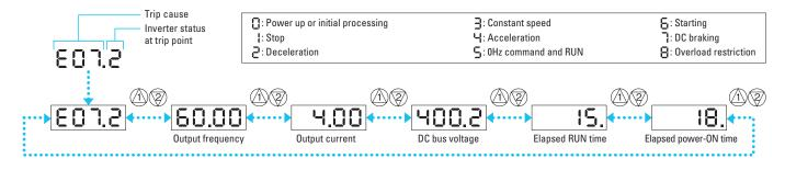
Note: Indicated inverter status could be different from actual inverter behavior. (e.g. When PID operation or frequency given by analog signal, although it seems constant speed, acceleration and deceleration could be repeated in very short cycle.)
