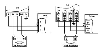
2) Wiring Drive, DB unit and DB resistor and DC reactor for SV750DB-4
