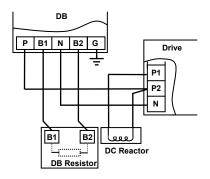
3) Wiring Drive, DB unit, DB resistor and DC reactor for SV2200DB-4
